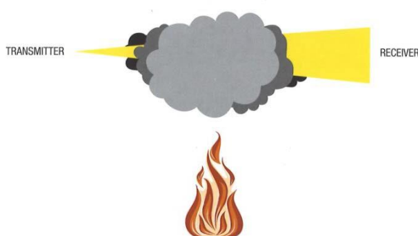
Figure 2: General Principle in Light Obscuration Photoelectric Alarms
