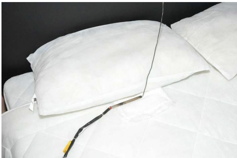
Figure 20: Visual Image of Cartridge Heater Placement on Bedding
