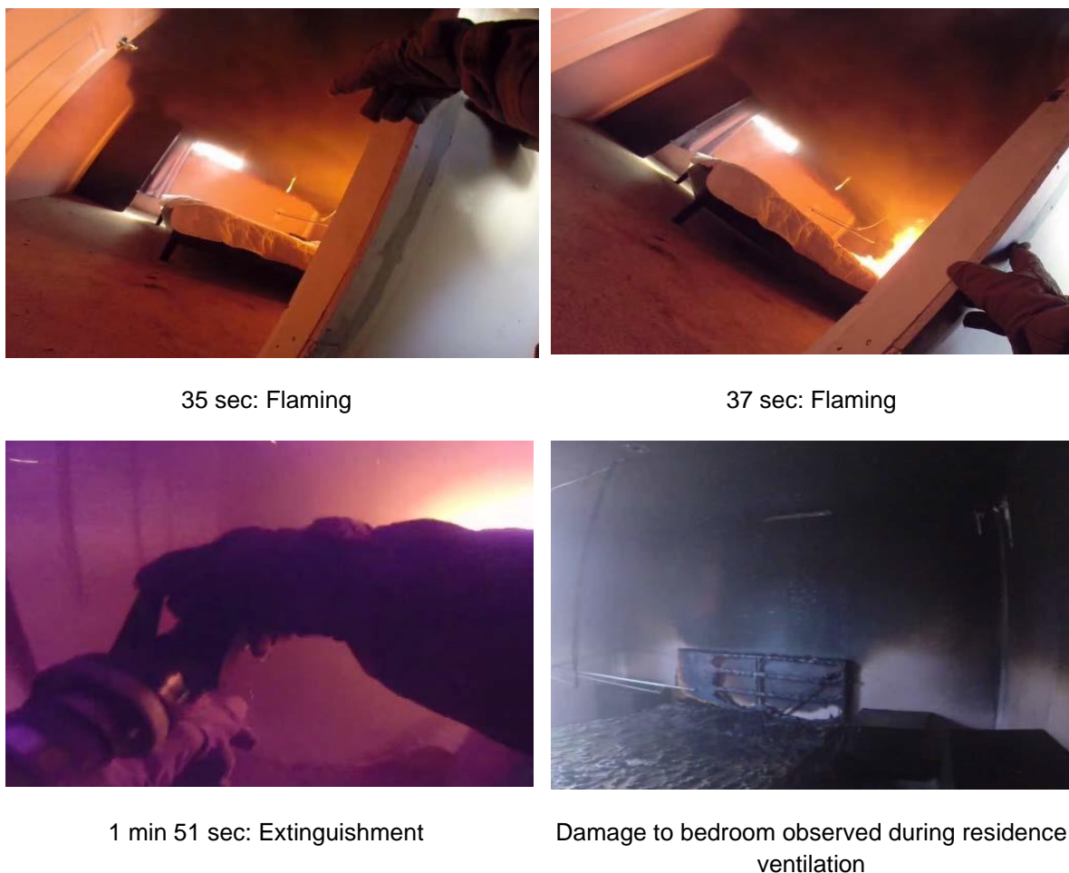
Figure 28: Burn 5 Images, Fire, Extinguishment, Damage
