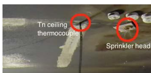
Figure 34: Burn 8 Tn Ceiling Thermocouple and Sprinkler Head Proximity
